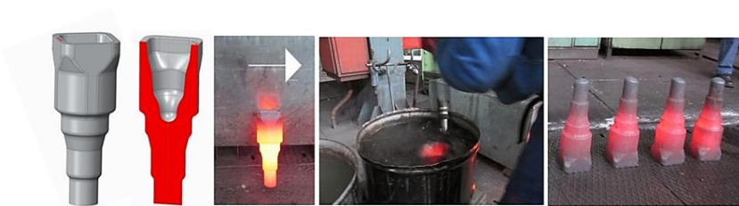
Figure 1. On the left side of the figure the forged spindle can be seen. On the right side of the figure the main stages of cooling process can be seen (starting point shown by arrow)
